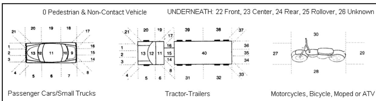
Record the number corresponding to the points of initial contact of Unit 1 and Unit 2 if applicable with another vehicle, person or object. If contact overlaps areas, more than one number should be recorded. For back distributed impact on an automobile, record “14, 15, 16.” Points of initial contact consists of parts which the vehicle first contacts, not secondary.
