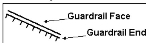
44 Guardrail Face in Median – A guardrail is a longitudinal barrier consisting of posts and rails or cables, whose primary functions are to prevent penetration and to safely redirect an errant vehicle away from a roadside or median hazard.
